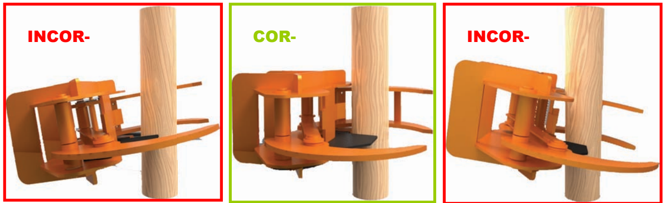
Figure 4. On the left, an upward slanting cutting position, and on the right, a downward slanting position. Both positions will place the blade under stress and can lead to the blade becoming damaged. The figure in the middle shows the correct position; the frame parallel with the tree.
